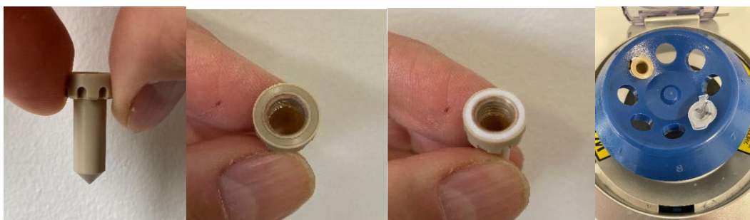
Figure 20: Sample vial. The groove should be clean and without dents and scratches. A new O-ring should be placed in the groove between each experiment.
