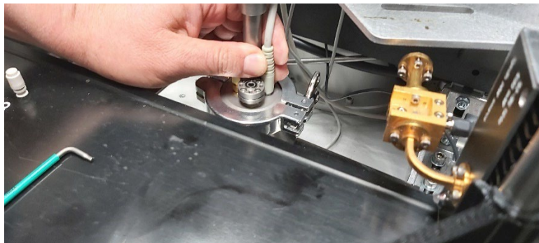
Figure 39 Disconnect probe temperature monitoring cable
