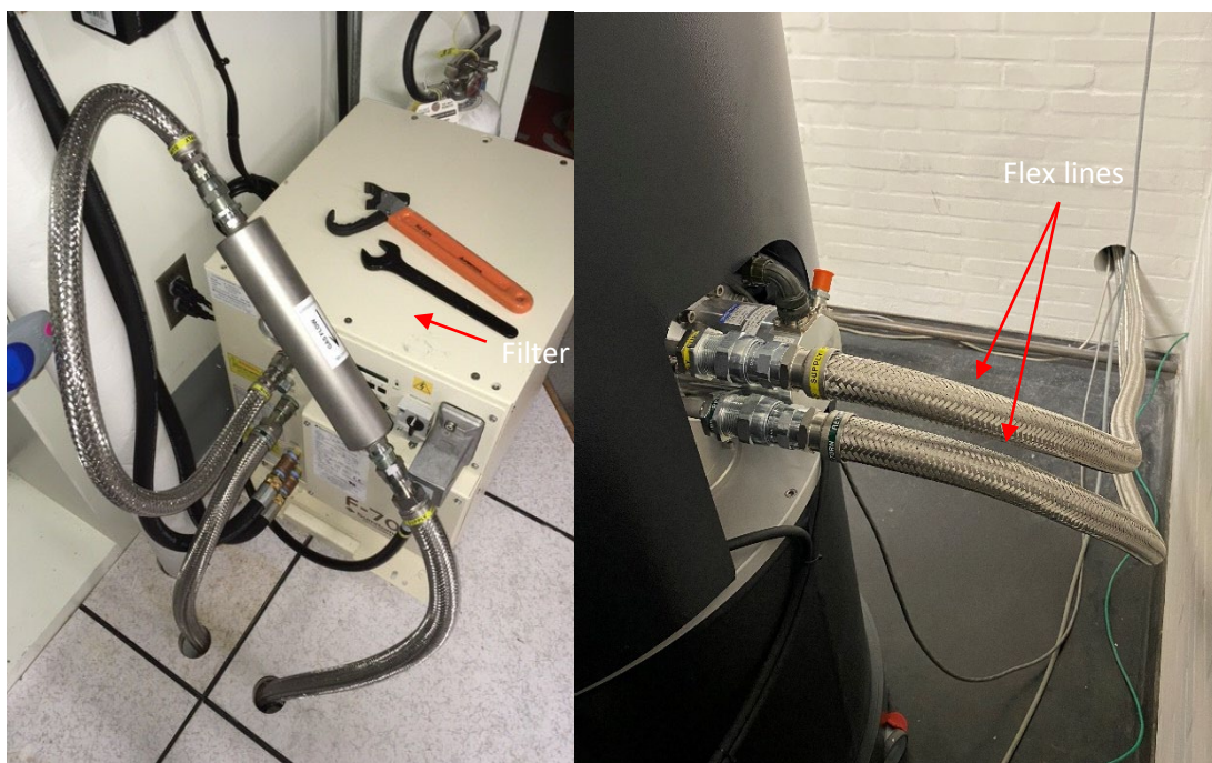
Figure 2: Left: F-70H compressor, flex lines and filter. Right: On the SpinAligner rear side the SRP082B cold head is connected to flex lines and a cold head control cable. The compressor is also connected to the SpinAligner by a USB serial communications cable.
