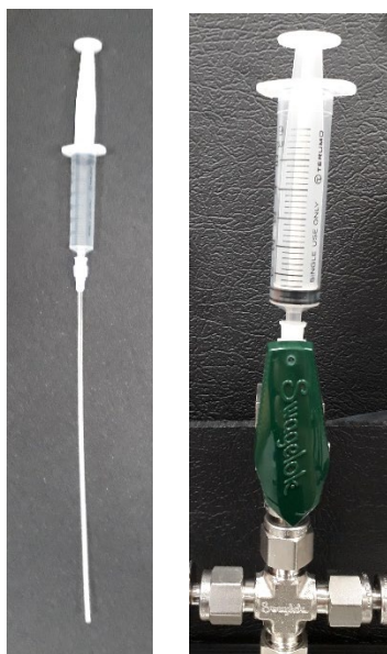
Figure 23: Syringe for loading dissolution medium.
