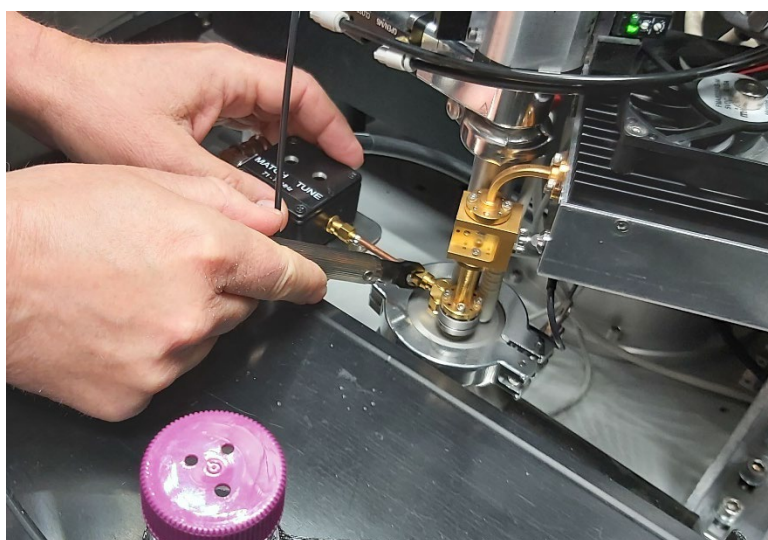
Figure 38 Unscrew Tuner & Match Box Coaxial cable
