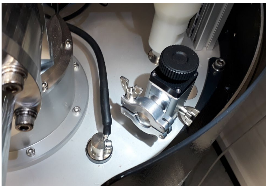
Figure 37: Enclosure KF16 pumping port.
